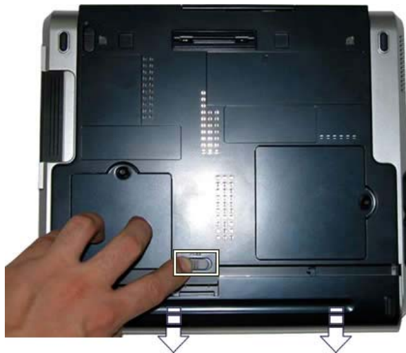
Fig. 1 Removing the Battery
